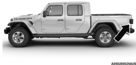
BSM Radar Location (Left Side Shown)
