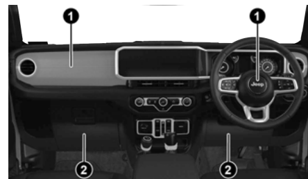
Front Air Bag/Knee Impact Bolster Locations
